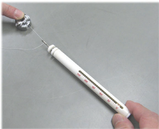
Upper/under thread tension measuring gauge Part name: UTG
